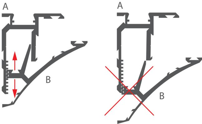
**8.** Place the shelf in the gap between the profile (B) and the mounting strip (A).
