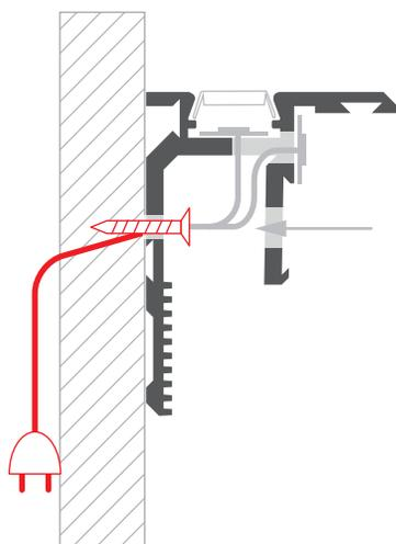
**6.** Insert the silicone string (F) into the the groove (B). Mount the extrusion (B) to the mounting strip.
