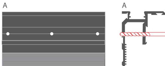
**2.** With a larger drill bit, widen the holes for the screws in the shorter wall of the mounting strip so that the heads of the screws can pass through.
