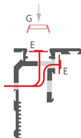
**5.** Screw the mounting strip to the surface and connect the power supply.
