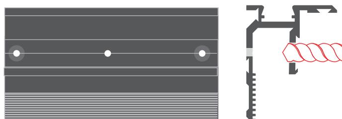
**3.** Drill a hole for the wires in the wall of the mounting strip at the same time the LED shelf approx. 8 mm long.
