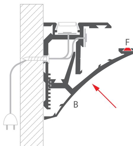
**7.** Positions of the extrusion(B) can be adjusted in 2 mm increments.
