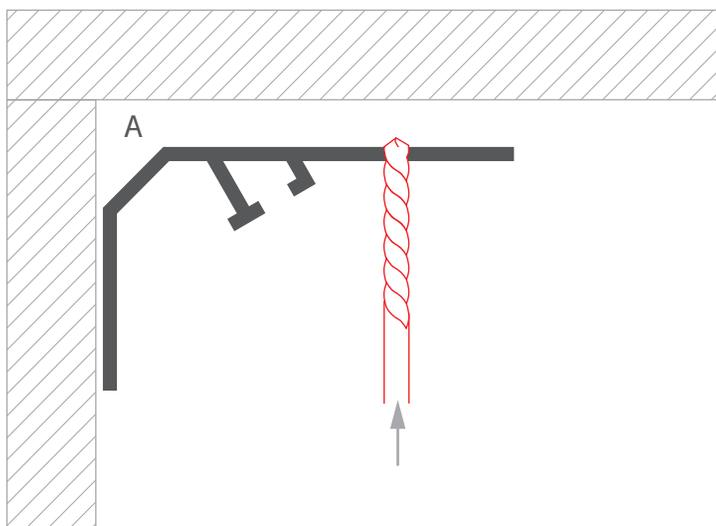
**2.** Attach the mounting strip to the mounting surface with suitable screws. Drill through the extrusion (B) to lead out the power cable.
