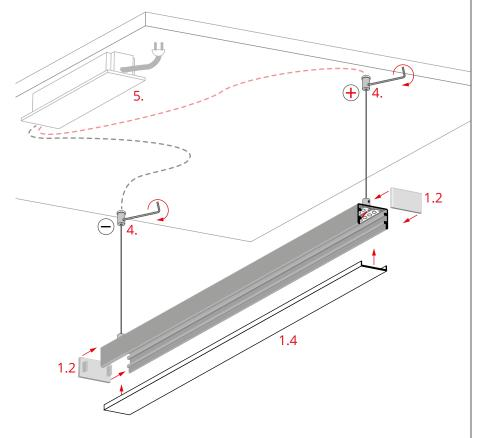
Mount the cover (1.4) and the end caps (1.2). Suspend the lighting fixture from the ceiling fasteners (4). Connect the 12V / 24V power supply (5) to the ceiling fasteners.
