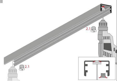
Chamfer the holes for threaded bolts (2.1).
