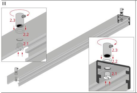
Insert the threaded bolts (2.1) into the drilled holes, put bases (2.2) on them and screw the heads (2.3) onto them.
