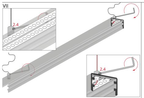
Lock the cables by tightening the pressure screws (2.4) in the heads of the fasteners.
