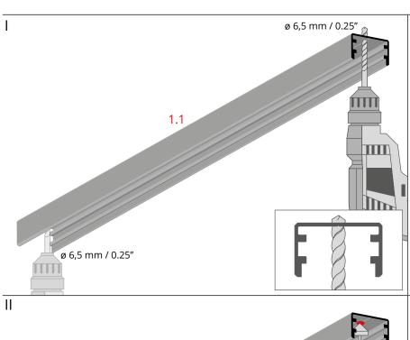
Drill holes in the profile (1.1) where the fasteners will be mounted.
