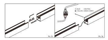
15.Connect lamps by connector, make sure both linear lights linked seamless, tighten the screws
