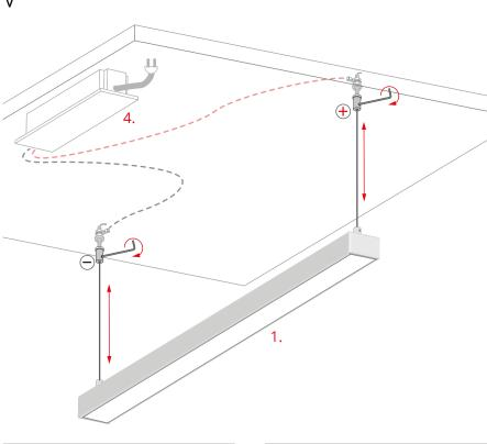
Suspend the fixture (1), adjust the length of the cables, so the fixture hangs evenly. Tighten the pressure screws (3.2) in the fastener bodies. Power supply cables must be connected to a 12 V / 24 V Power supply (4).
