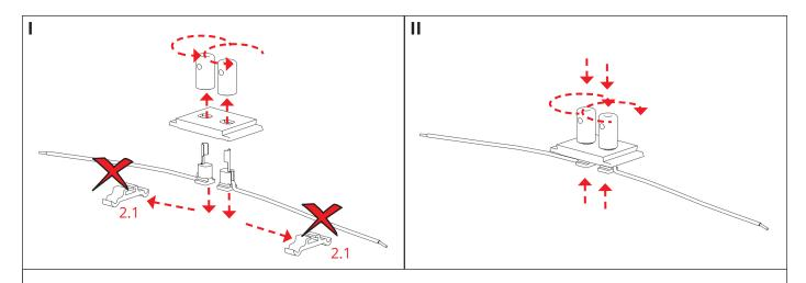
In case of installation in the GIZA-DUO-LL profile, unscrew the fastener and remove its blockades. Then fold the fastener back.
